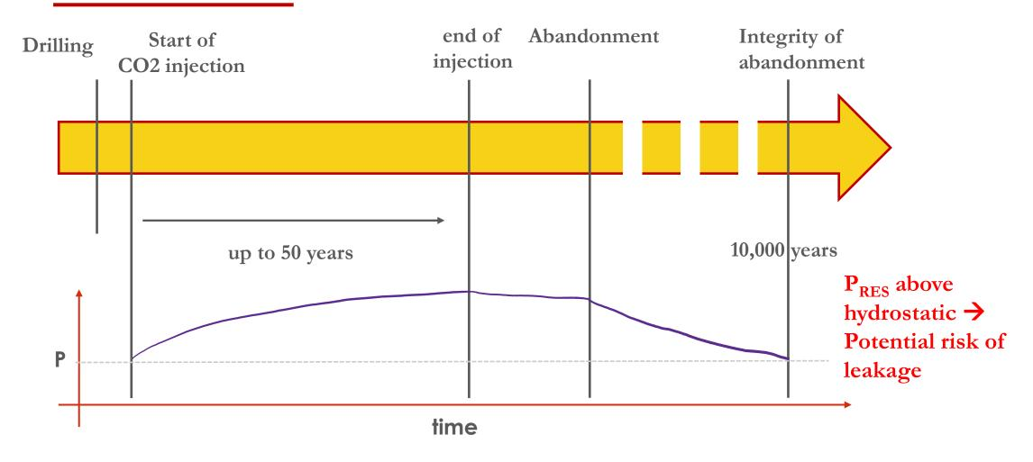
Reservoir pressurization due to CO2 injection
